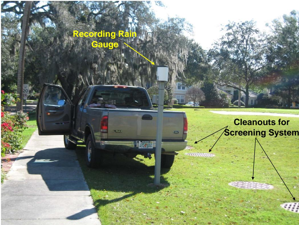
**Figure 2-9. Recording Rainfall Collector.**
